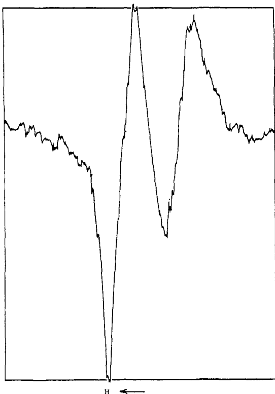
Figure 1. F^{19} nmr spectrum of 50 vol % solution of " O_3F_2 " in OF_2 .
